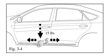
(d) Use a lint free cloth and apply even hand pressure to adhere the lower rocker molding to the vehicle (Fig. 3-4).
